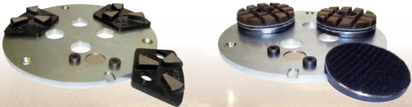
Kut-Rite's new Quick Disconnect tool mounting design is redefining how diamond tools are mounted. The QD system incorporates two locating pins, for precise tool positioning and the use of powerful neodymium rare earth "super magnets" to hold the tools in place. The result of this combination produces a tool system that allows quick and precise placing of tools for smooth running, holding power that virtually eliminates tool kick out during operation and extremely fast removal/insertion time.
