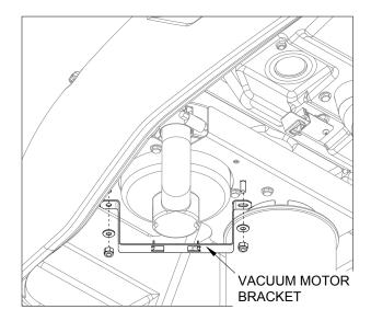
7. Remove three (3) screws that secure vacuum motor assembly in place. Remove vacuum motor assembly, as shown below.
