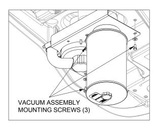
8. Remove move three (3) screws that secure vacuum motor. Replace motor.
