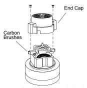
If armature commutator is grooved, extremely pitted or not concentric, the motor will need to be replaced or sent to a qualified service center.
