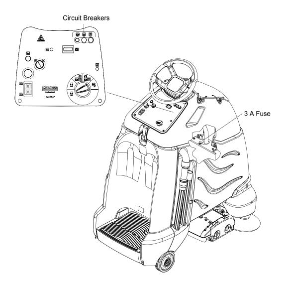
Circuit breakers interrupt the flow of power in the event of an electrical overload. When a circuit breaker is tripped, reset it by pressing the exposed button. If a circuit breaker continues to trip, the cause of the electrical overload should be found and corrected.
