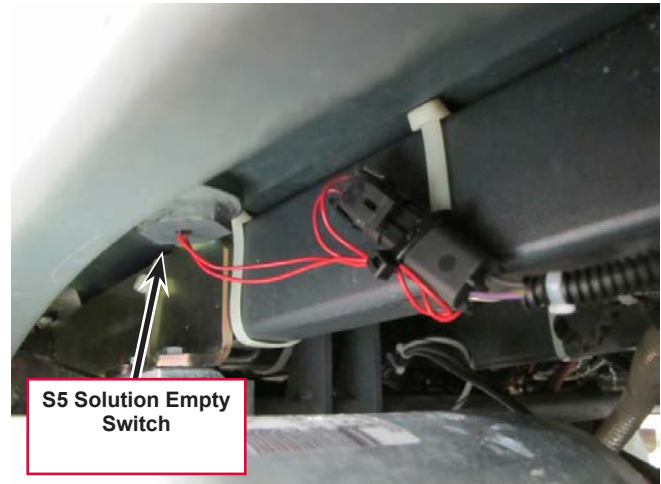
Viewed from under solution tank
