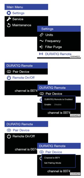
Now, continue with the grinder. Press the *Main menu* button, and select using the arrow keys *DURATIQ Remote* respectively.
