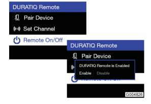
Go to Set Channel respectively. Each grinder/dust extractor pair needs to have its own channel for communication. Select a channel with the arrow keys and press OK.
