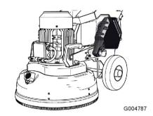
Disconnect the motor cable. Make sure that the chassis does not fall backwards when you then remove the pins holding the grinding head.
