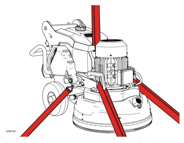
Always make sure that the machine is securely anchored to its surroundings and that the grinding head is lowered on to the surface. Tighten the securing straps, or other equipment used for anchoring during transport over non-moving parts, e.g. the machine's chassis.
